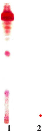
Figure (5): TLC chromatogram showing results of using Nicloux reagent with hashish sample (0.5g) for 2 minutes (1) Control, (2) Treated sample. The mobile system was chloroform: benzene (7:3) and TLC was developed with fast blue as developing reagent.
